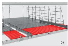
Repeat these steps bay by bay. Reposition the rearmost roller unit onto the front-most transverse beam (see step 3). Secure all components with a pin.
